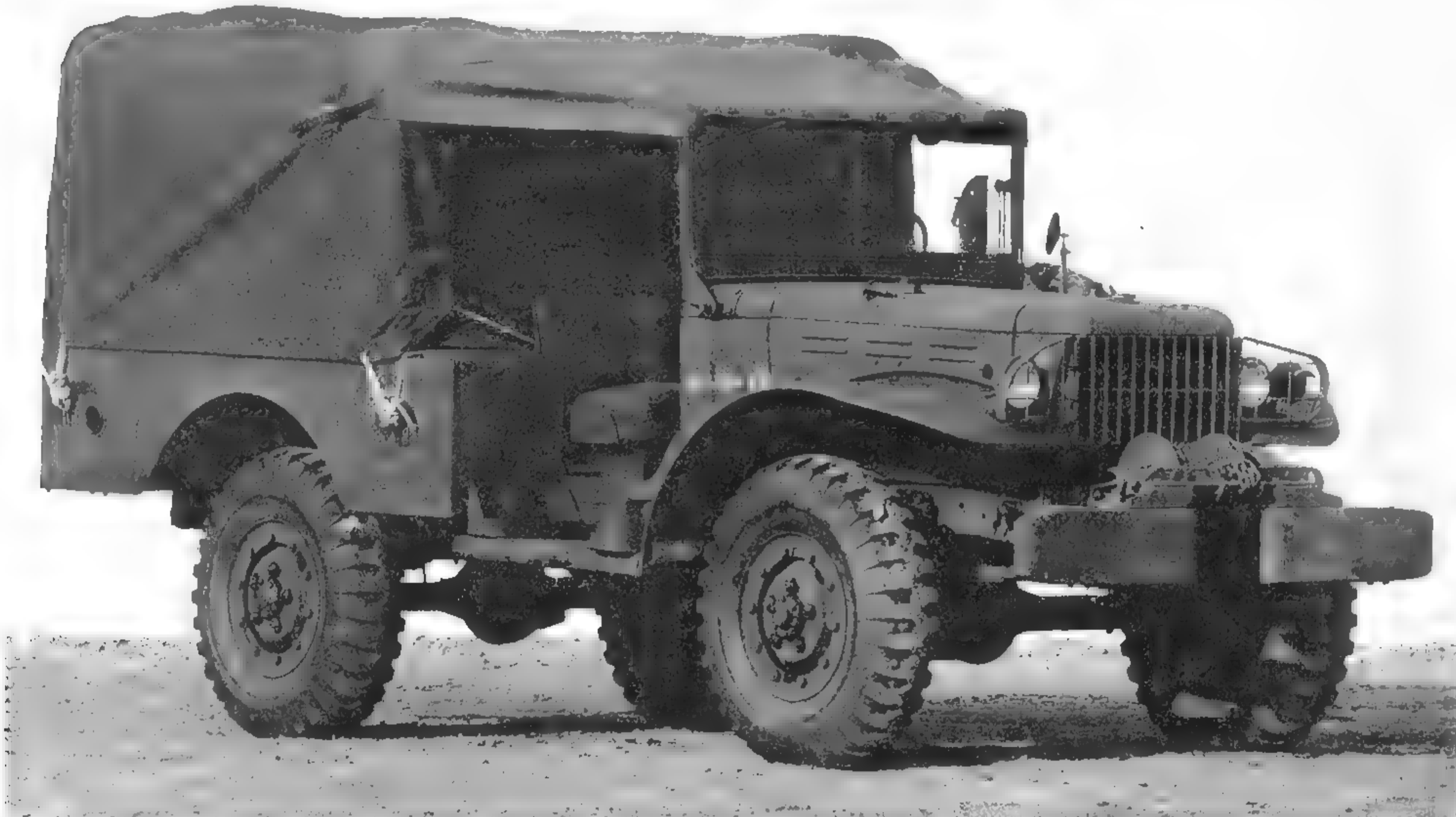
This photo was taken at the Studebaker Proving Grounds in January 1944, and shows the typical Dodge WC-52. The Braden PTO-driven winch is visible, as is the large one-piece canvas that covers both the driver's and cargo compartment. (U. S. Army photo)
